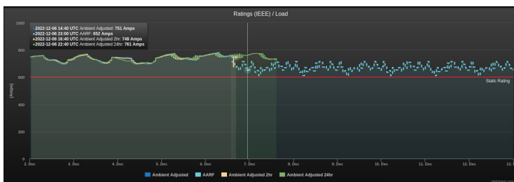
Figure 1: SMARTLINE AAR/881 provides a simple visual display of all 240 1-hour line ratings for each line.
