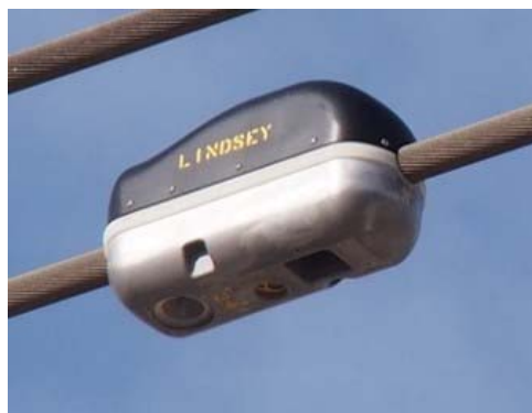
Figure 3: Self-contained next generation DLR conductor monitor with built-in magnetic field harvesting power supply, communications, LiDAR, current sensing, and temperature sensors.
