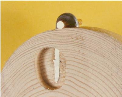
Sectioned example of fishhook staple shows holding power of patented fishhook design.
